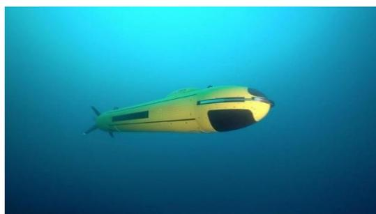
Autonomous Underwater Vehicle (AUV) A18-M
